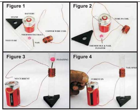
**Materials Require :** A test tube, Thermocol ball, 1.5 volts battery, Copper wire, Pin (Nail). A triangular piece of sponge. You can also take a piece of Thermocol instead of a sponge.
